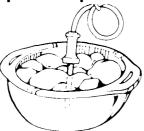
For casseroles, the tip of the probe should be in the center of the food. Stir foods when recommended. Replace the probe.
